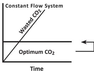
One of the unique features of our system is its ability to raise the CO<sub>2</sub> up to the appropriate level each day when your lights come on and then maintain it. CO<sub>2</sub> is an essential ingredient for photosynthesis, which is the main provider of energy for plant growth. Without enough carbon dioxide, plant growth will slow down or can actually stop. A lack of CO<sub>2</sub> can occur very easily in an enclosed growing area unless you add a supplemental source of CO<sub>2</sub> gas.
