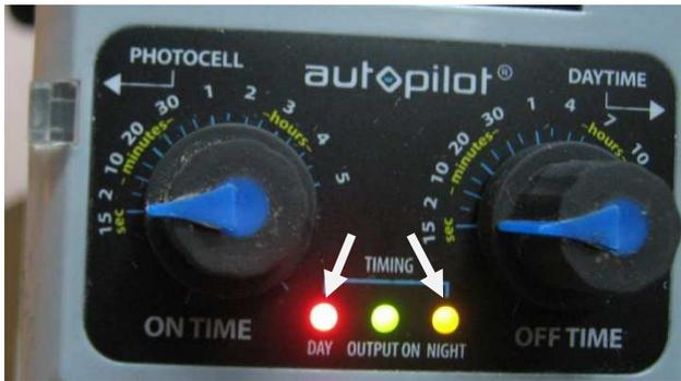
Plug a small device into the outlet. When the OUTPUT ON light (green LED) comes on, the outlet should have power.
