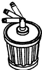
6. Do not immerse the emitter or ionizer in water or detergents. When the emitter pin becomes dusty, it may be cleaned with a cotton swab and vinegar.
